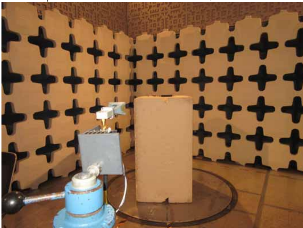
Test Setup for Radiated Emissions – 18GHz to 26.5GHz, Vertical Polarization
