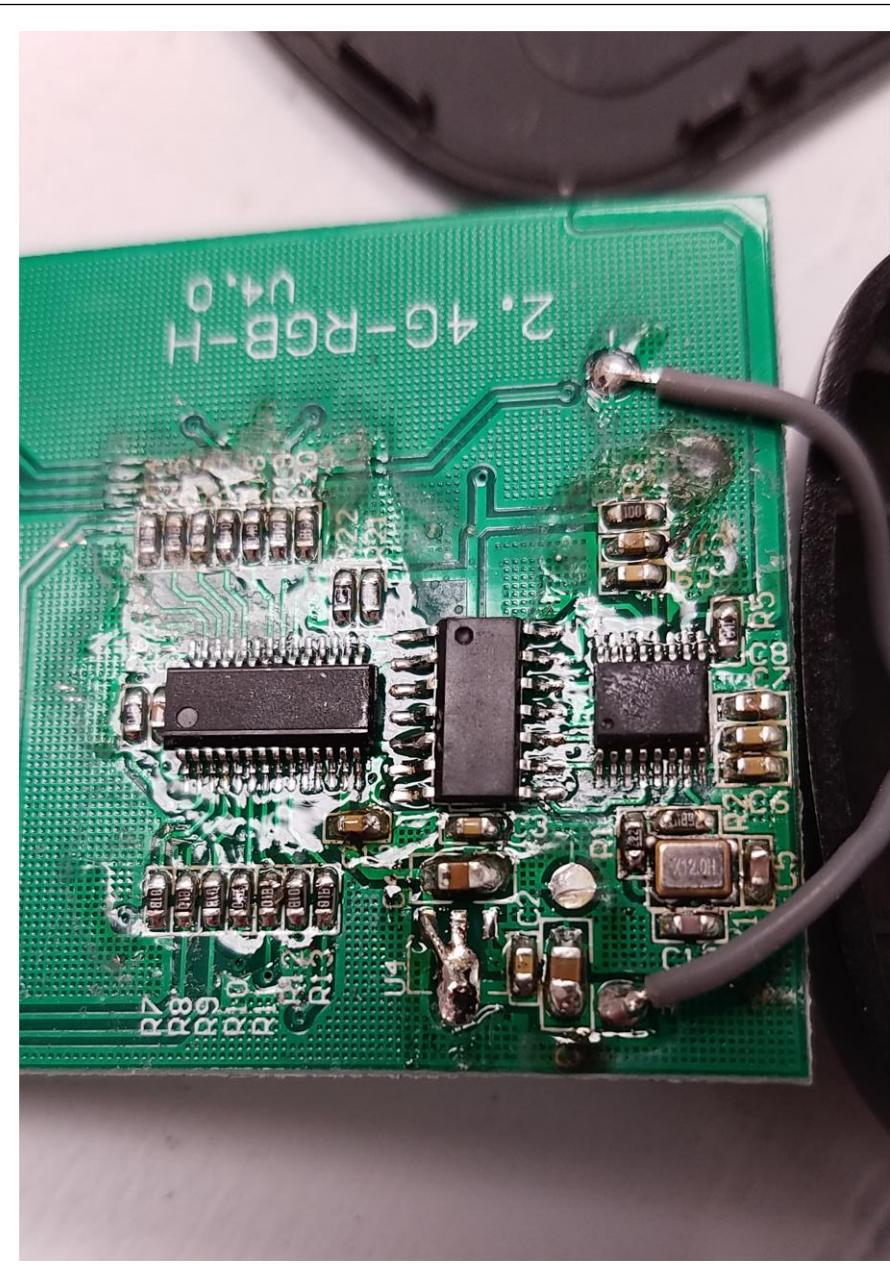
The RF chip installed on the controller, Model # LT8900, is produced by Idctek company. EIKO obtains this chip is through the agency-Shenzhen JMRTH TECh Co. Ltd. under JMRTH's Model #: JMR10P370. For confidential purposes, the identity of the RF chip is masked.
