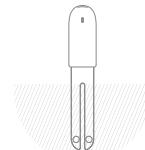
Please make sure at least 2/3 of soil moisture sensor sectionbe inserted into the soil
