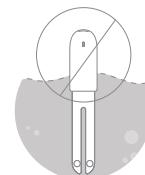
Never immerse the sectionabove moisture sensors in water
