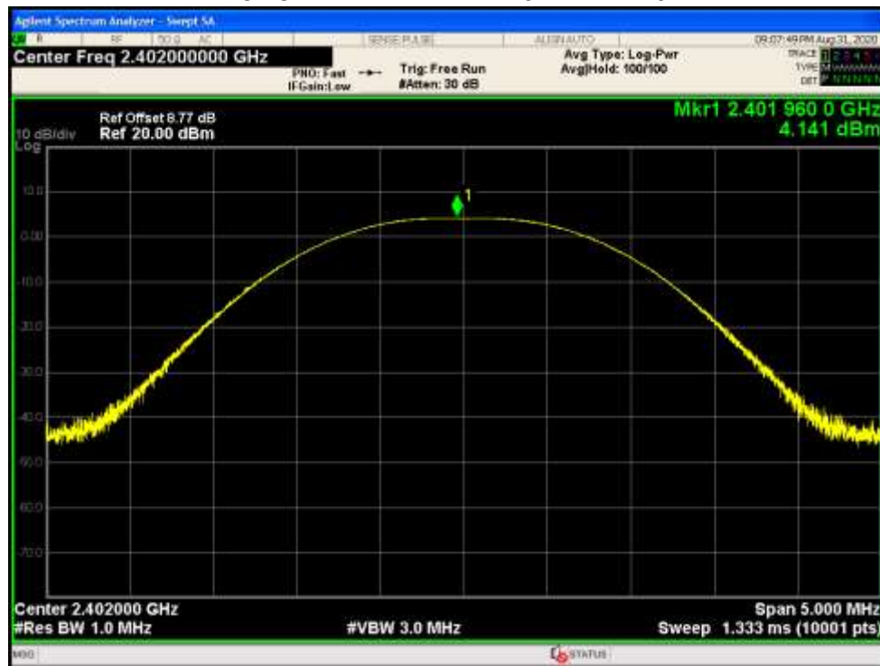
Power NVNT 1-DH1 2402MHz Ant1
