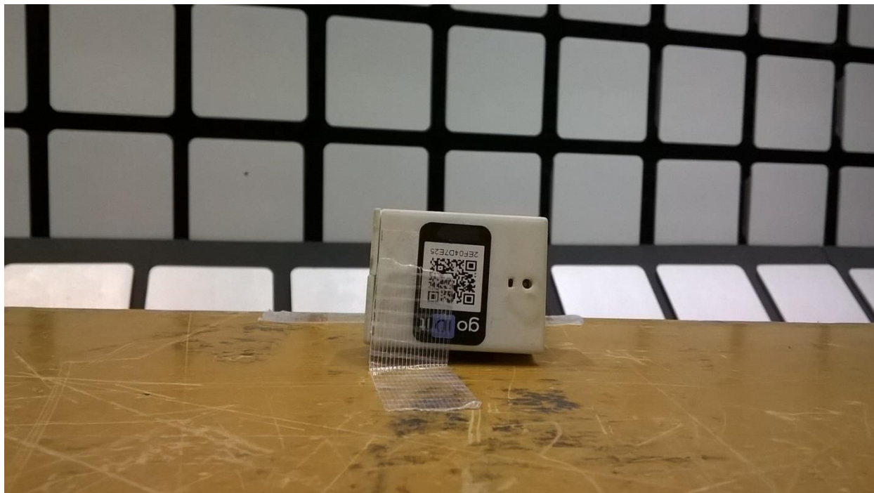
Figure 5 - Test Setup for 1 - 25 GHz, Horizontal Orientation
