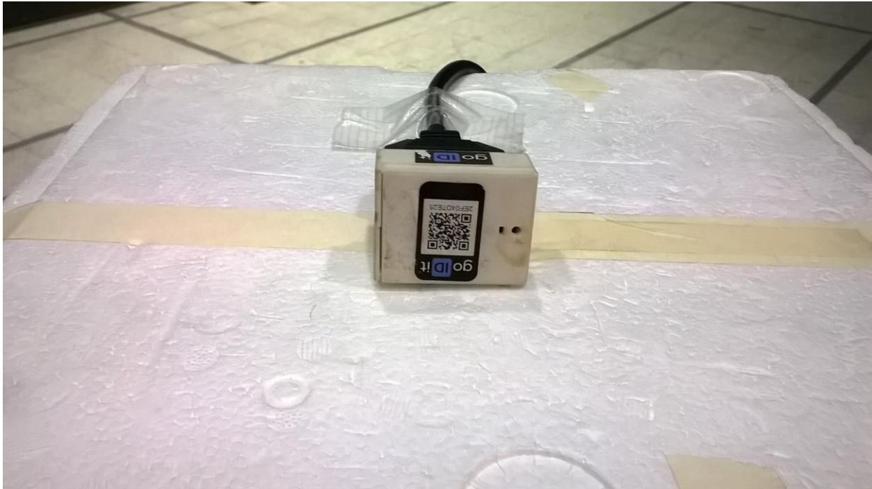
Figure 1 - Radiated Emissions Test Setup, X-axis
