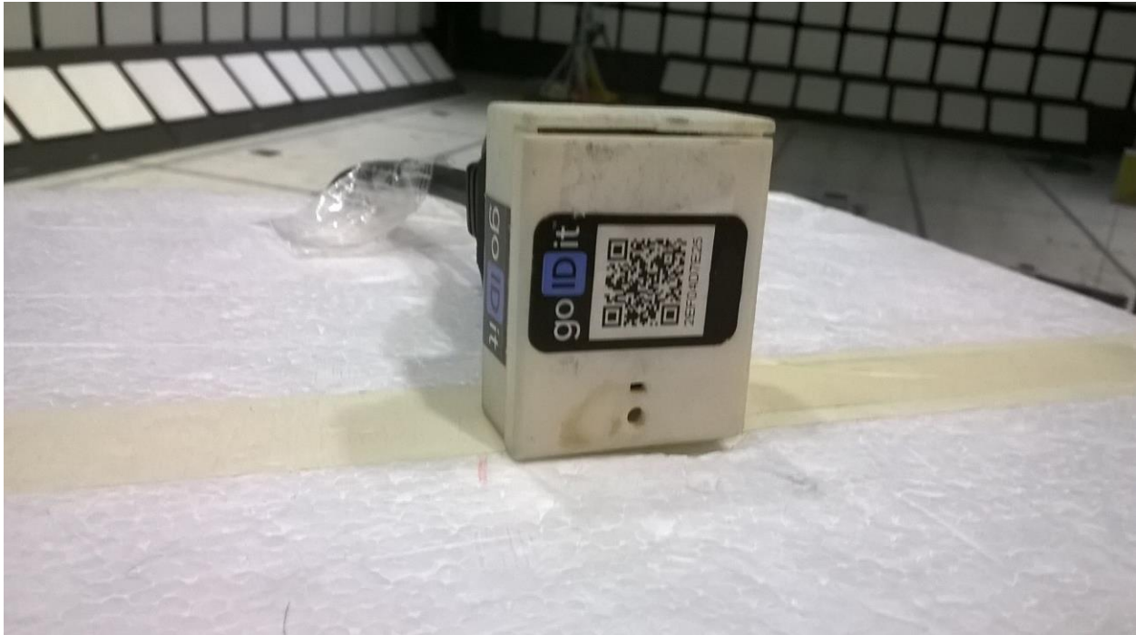
Figure 3 - Radiated Emissions Test Setup, Z-axis
