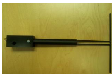
Figure 1 – MVG COMOSAR Validation Dipole
