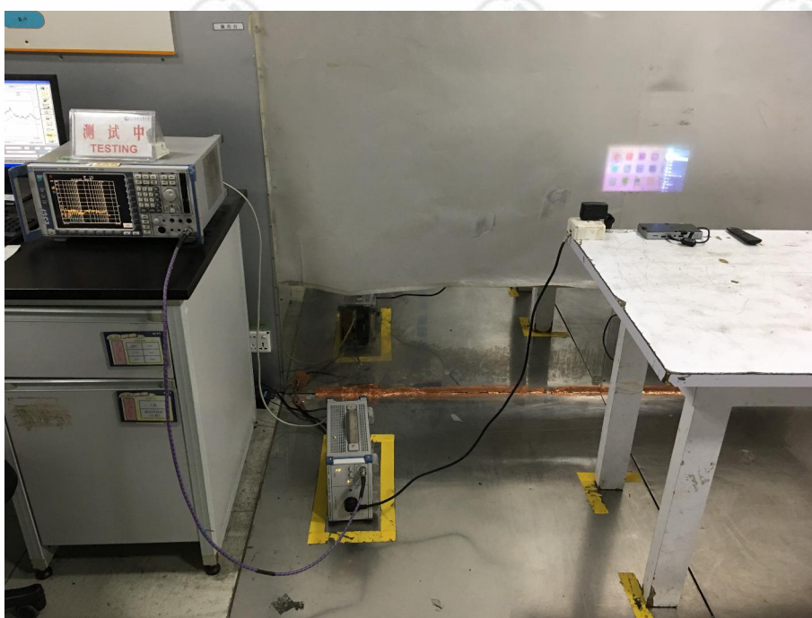
Conducted Emissions Test Setup
