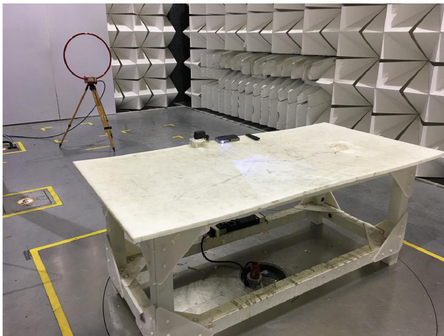
Radiated spurious emission Test Setup-1(Below 30MHz)
