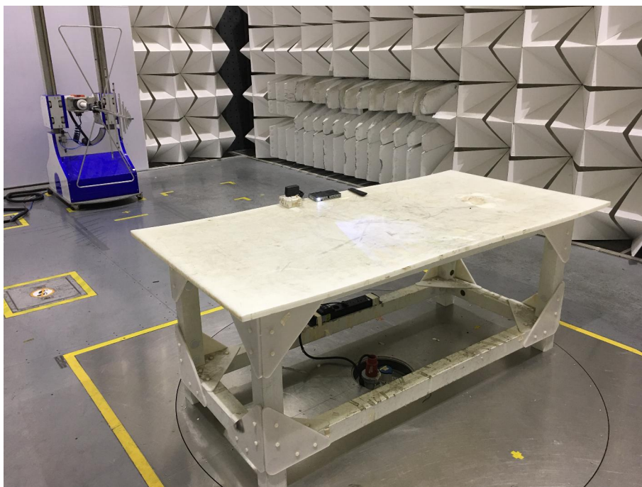
Radiated spurious emission Test Setup-2(30MHz-1GHz)
