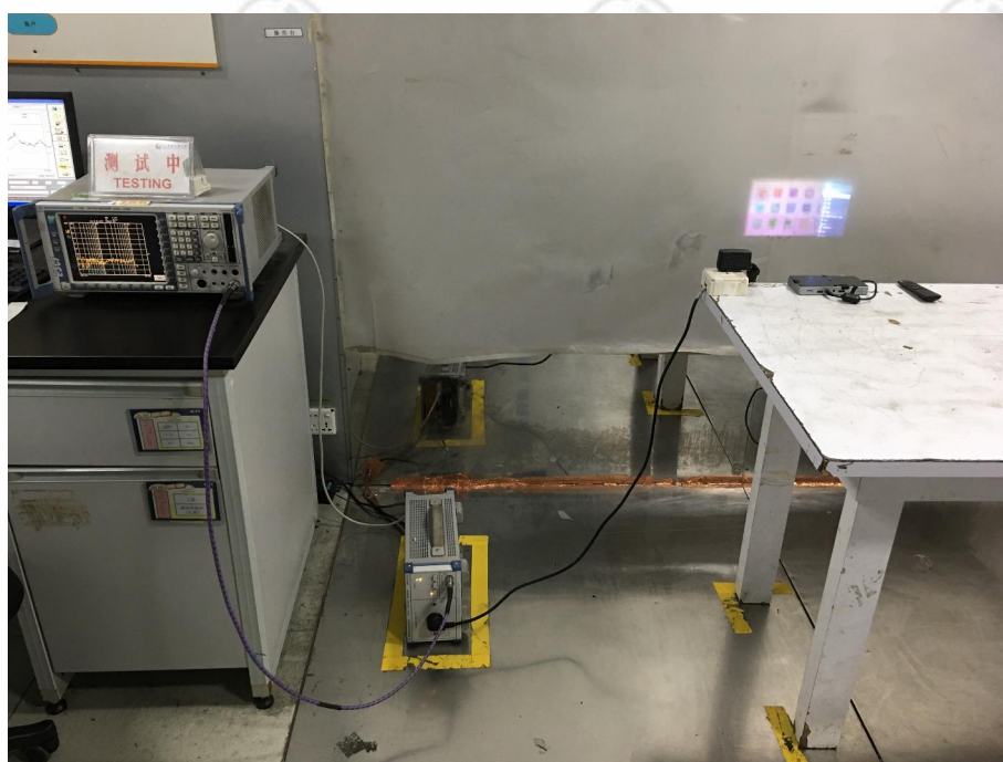
Conducted Emissions Test Setup
