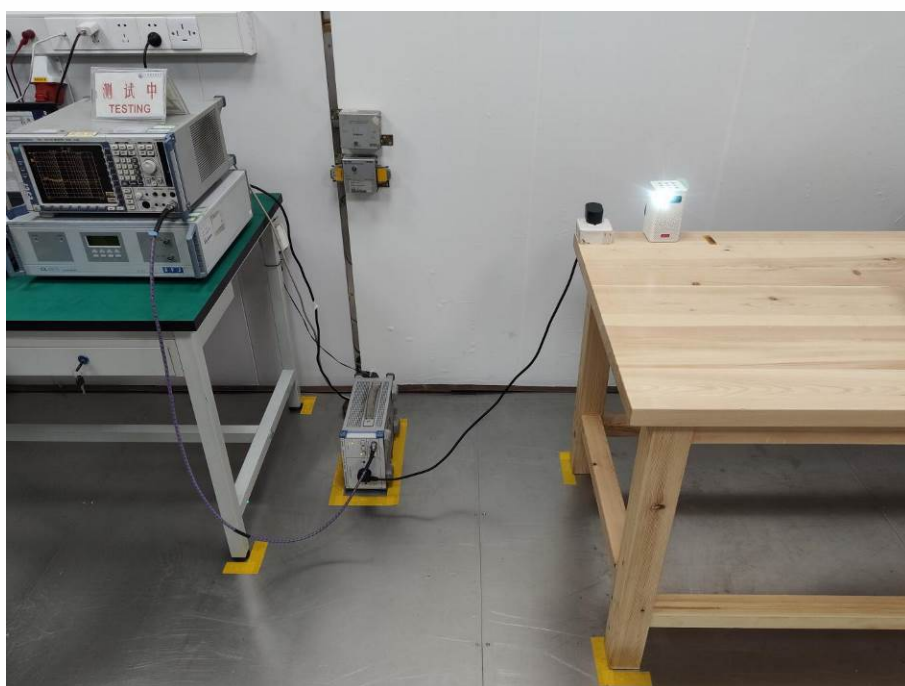
Conducted Emissions Test Setup
