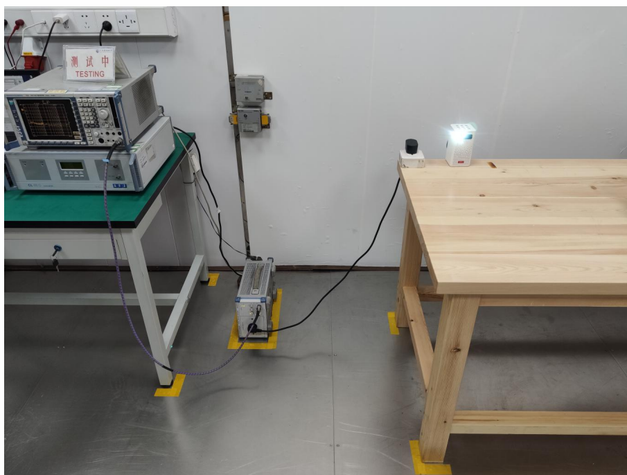
Conducted Emissions Test Setup
