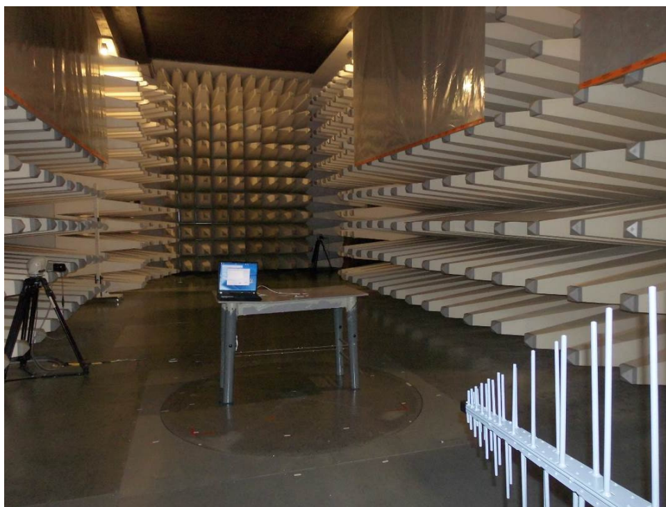
Set-up for Radiated Emission
