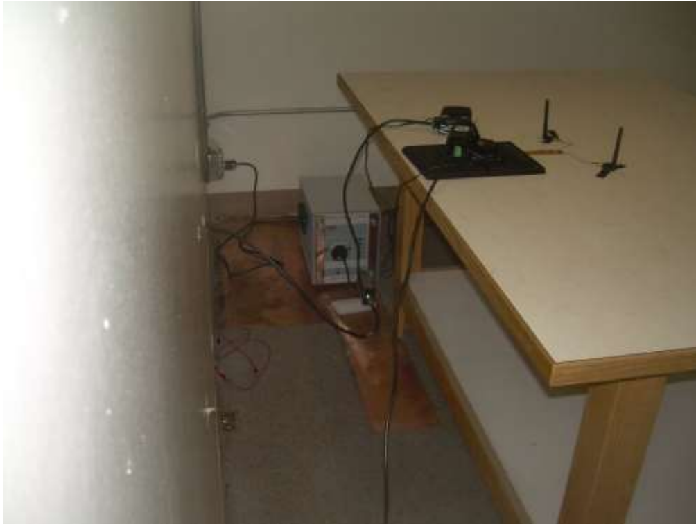
Photograph 9: Back View Conducted Emissions Worst-Case Configuration
