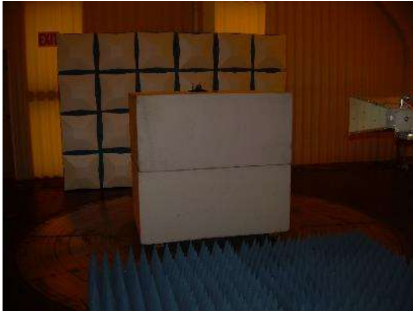
Photograph 3: Front View Radiated Emissions Worst-Case Configuration (Module Flat and Antennas Vertical) – Above 1000 MHz
