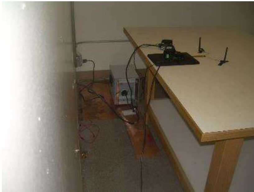
Photograph 9: Back View Conducted Emissions Worst-Case Configuration
