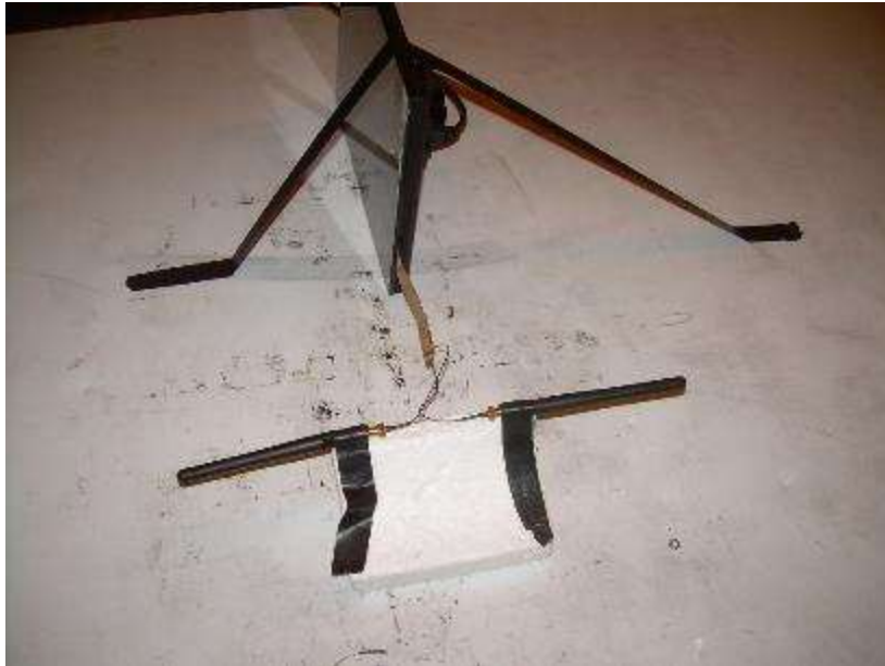
Photograph 5: View Radiated Emissions Module On Edge and Antennas Horizontal
