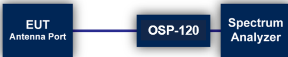
Figure 2: Direct Connection at the Antenna Port Test
