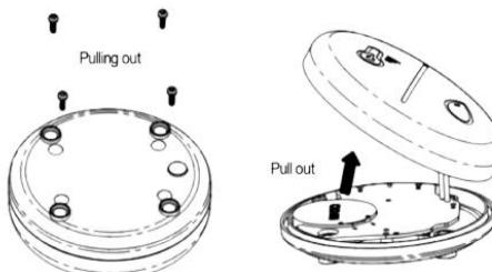
3. **Replace the Battery:** Carefully remove the old CR2450 3.0V (600mAh) battery and insert a new one, ensuring the positive (+) side is facing up.
