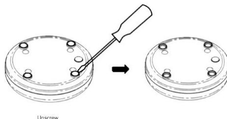
2. **Remove the Battery Cover:** Unscrew the screws from the plastic casing and gently lift the front cover to reveal the battery compartment.
