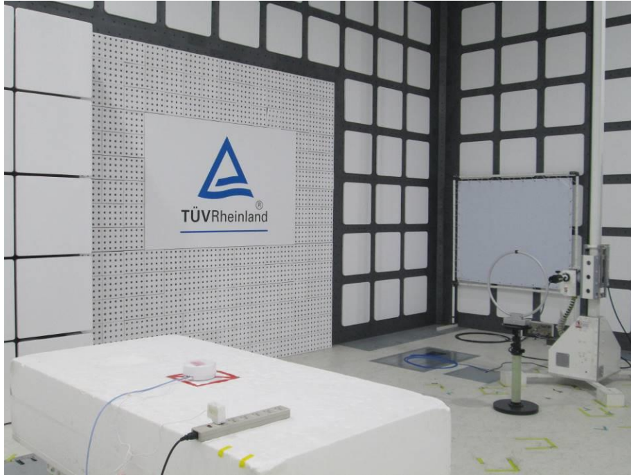
Photograph 4: Test Setup for Spurious Emissions (Back View 2)
