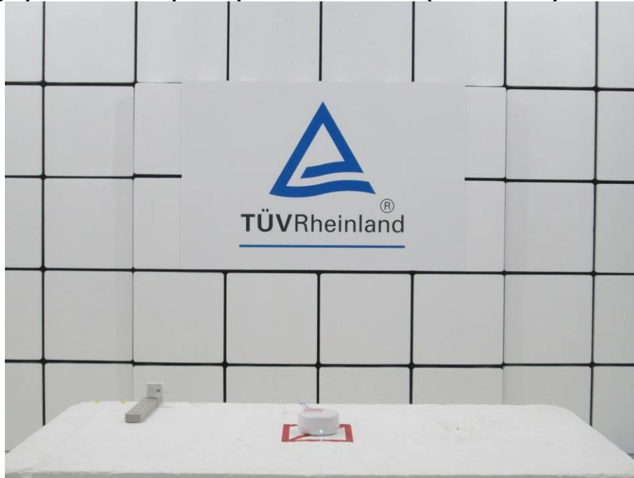
Photograph 1: Test Setup for Spurious Emissions (Front View 1)
