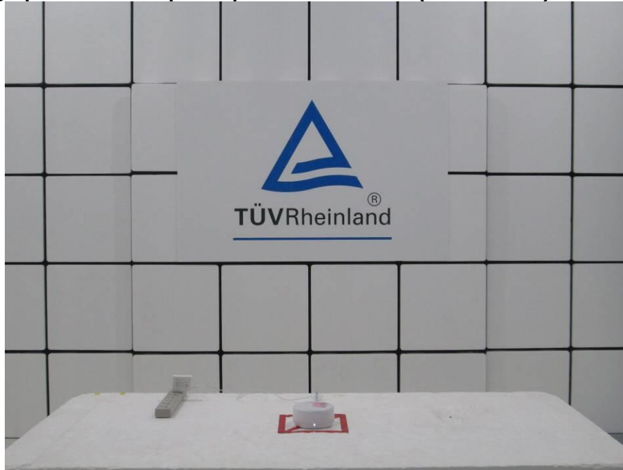
Photograph 10: Test Setup for Spurious Emissions (Back View 1)
