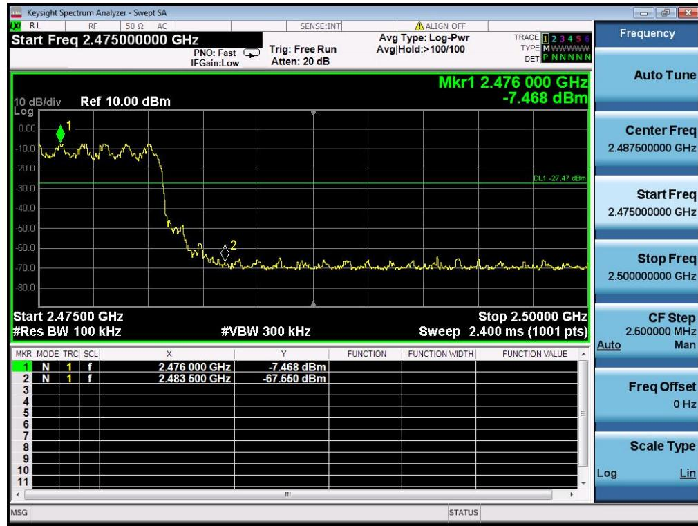
EDR mode(8DPSK): Band Edge-Left Side
