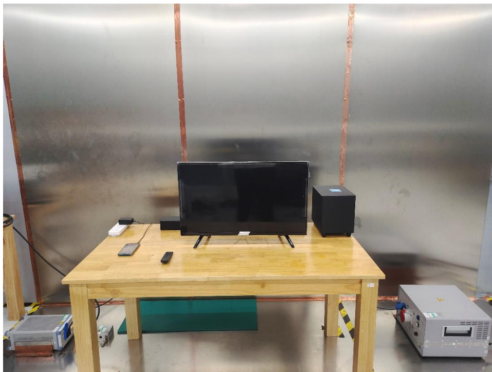
Photograph 3: Set-up for Conducted Emission on AC Mains
