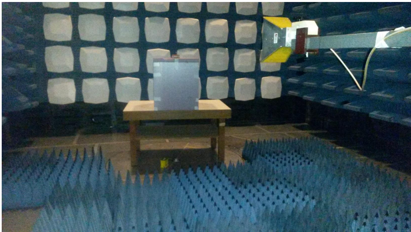
Radiated Emission test setup in Semi Anechoic Chamber
