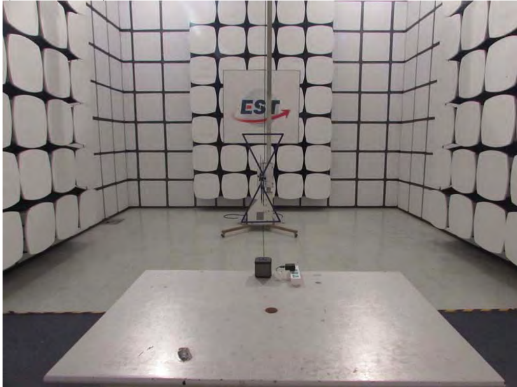
Radiated Test (30-1000 MHz)
