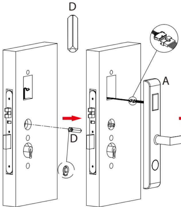
**7. Install spindle (C) and (D)**
