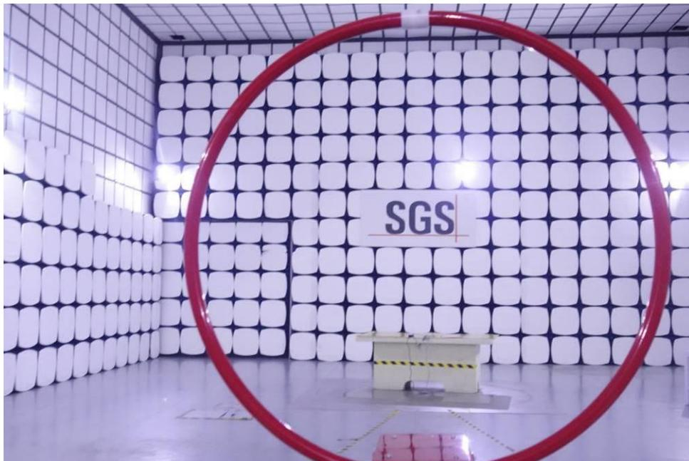
**1.4 Radiated Emissions(30MHz-1GHz) Test Setup**
