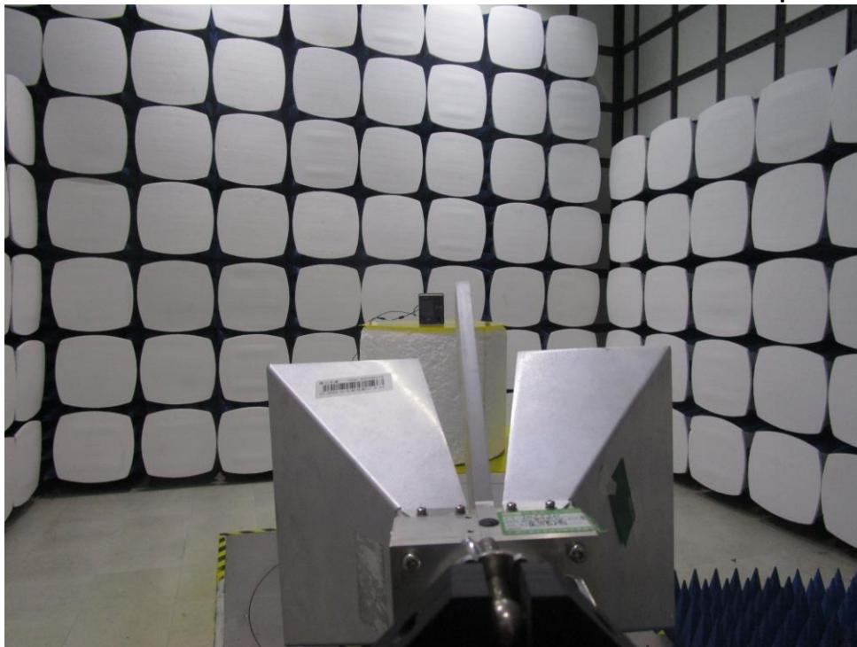
**1.3 Radiated Spurious Emissions Test Setup**
