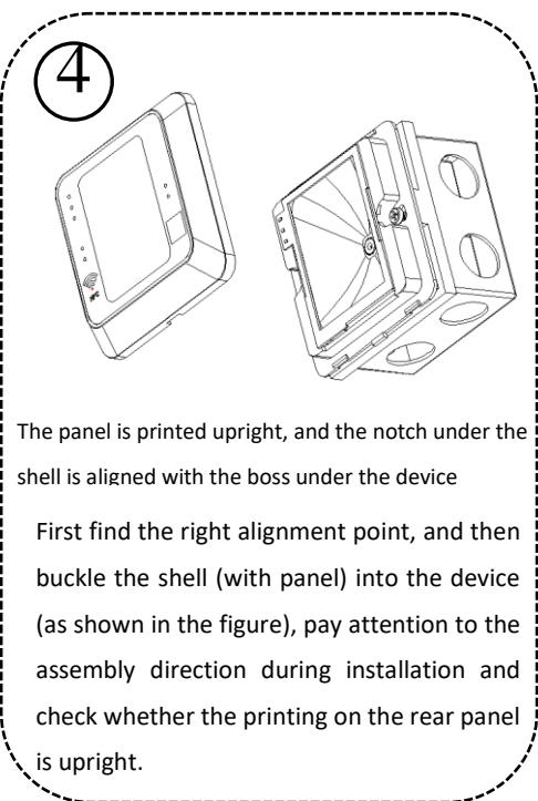
The panel is printed upright, and the notch under the shell is aligned with the boss under the device
