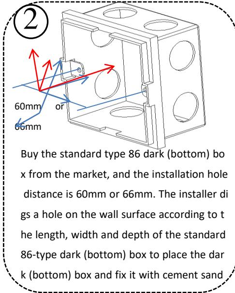
Buy the standard type 86 dark (bottom) box from the market, and the installation hole distance is 60mm or 66mm. The installer digs a hole on the wall surface according to the length, width and depth of the standard 86-type dark (bottom) box to place the dark (bottom) box and fix it with cement sand.
