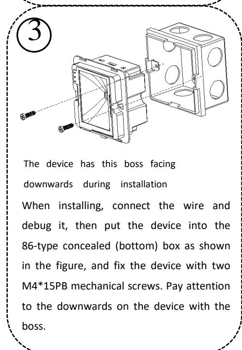
The device has this boss facing downwards during installation
