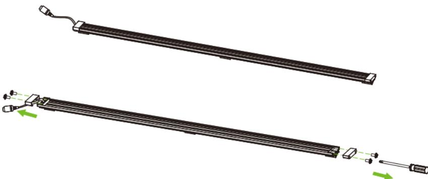
**Step 2:** Position the device with its back facing the guideway, snap it onto the guideway, and slide it towards the center. This setup supports the installation of multiple devices.
