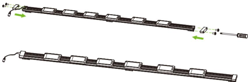
**Step 4:** Snap the terminals of the power connection cable vertically onto the magnetic conductive strip.
