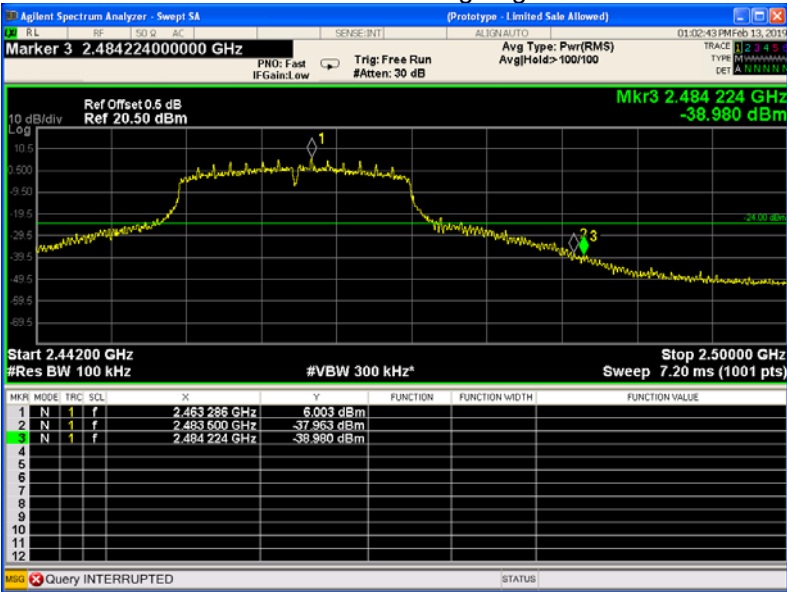
TX 11n HT20: Band edge-right side
