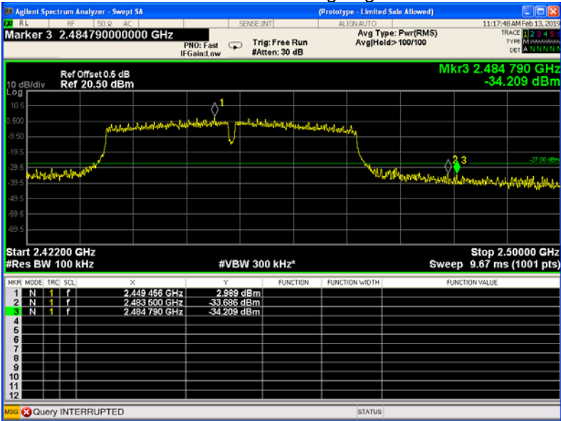
TX 11n HT40: Band edge-right side
