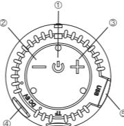
1. ON/FF button: Long press to turn Power ON/OFF; Short press for Play / Pause; Short twice press to switch to FM mode; Short press to enable automatic search in FM mode.
