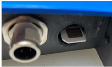
Figure 34 SIM card installation
