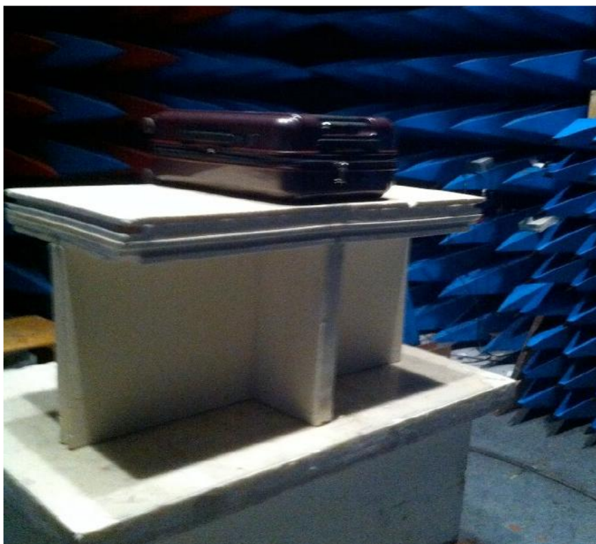
Radiated emissions measurements setup above 1GHz
