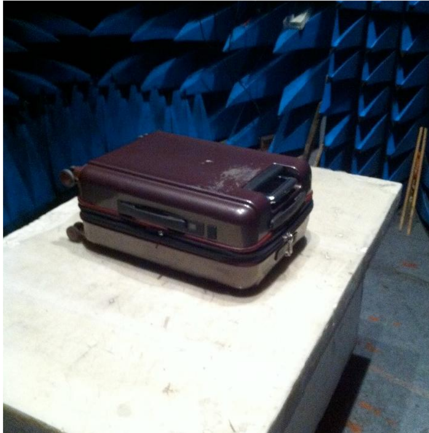
Radiated emissions measurements setup below 1GHz
