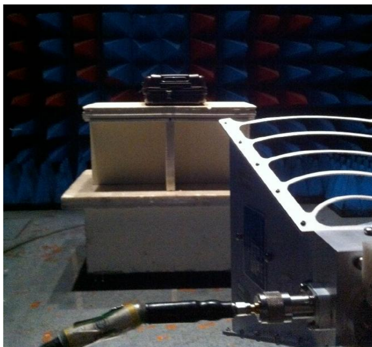
Radiated emissions measurements setup above 1GHz
