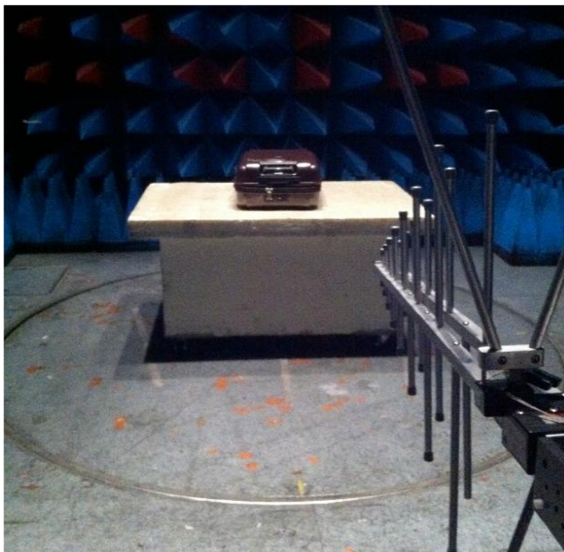
Radiated emissions measurements setup below 1GHz
