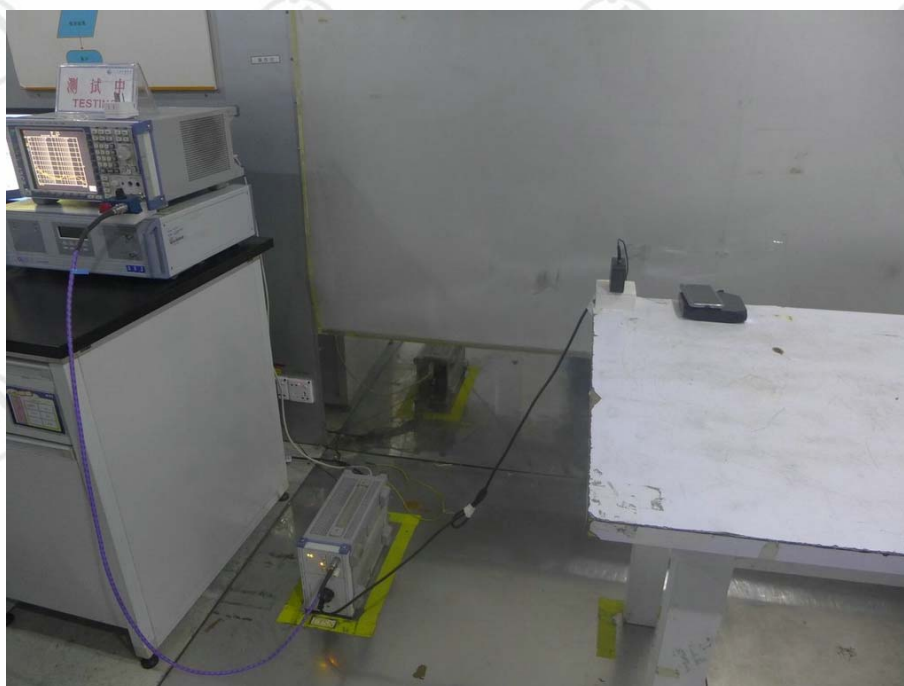
TEST SETUP OF CONDUCTED EMISSION
