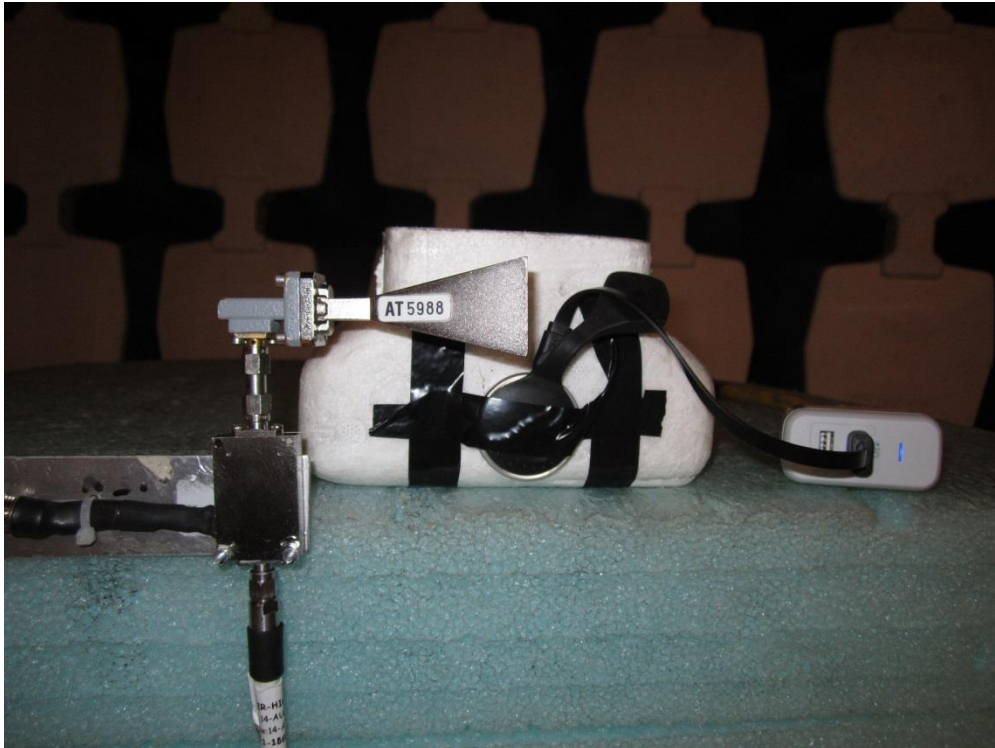
Radiated Emissions - 18 to 25 GHz
