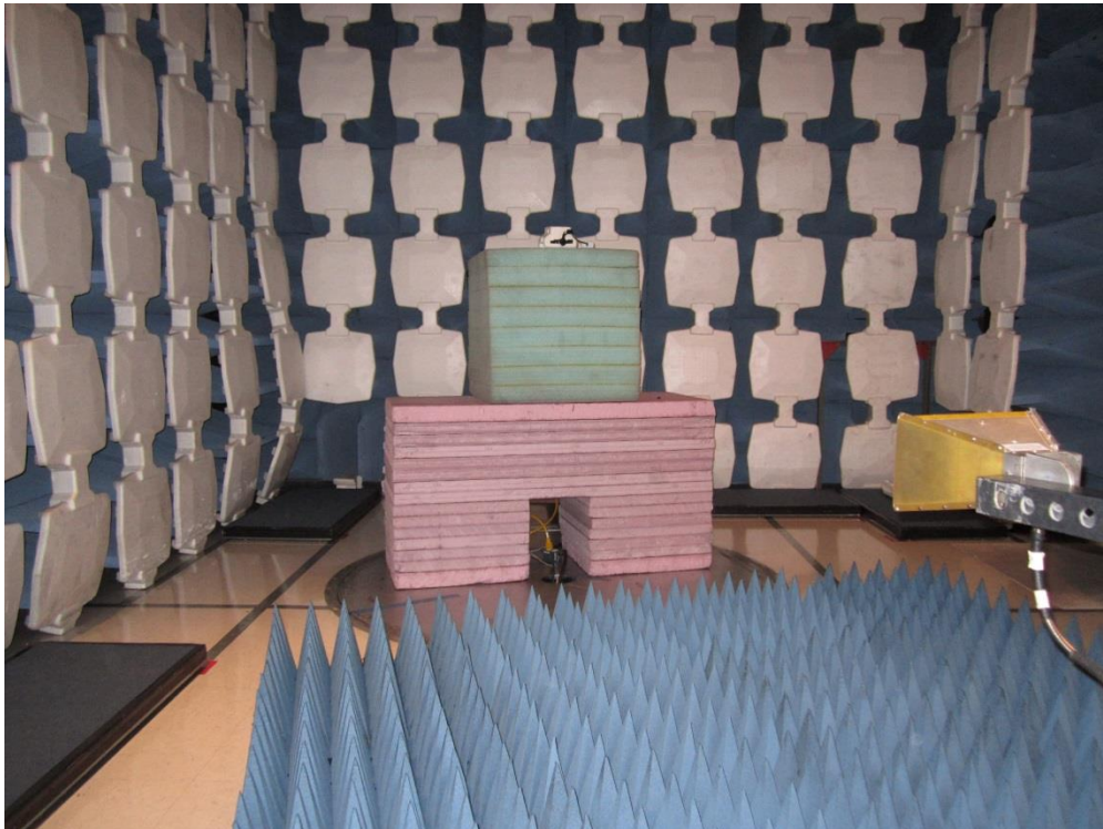
Radiated Emissions - 1 to 6 GHz
