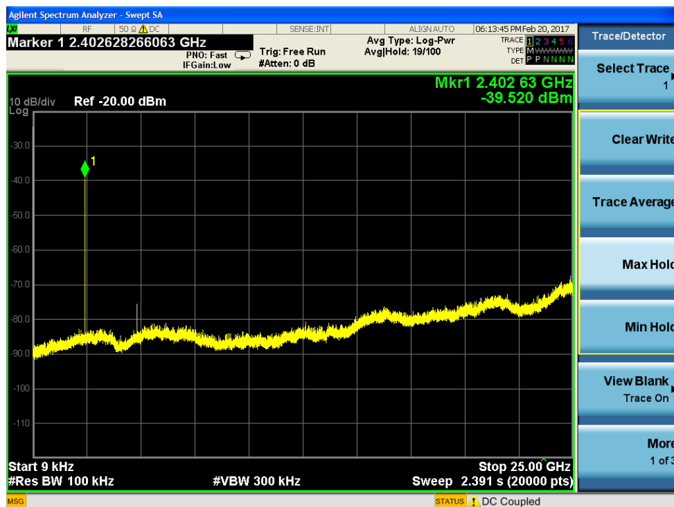
Low Channel 9 KHz -25GHz Conducted Spurious
