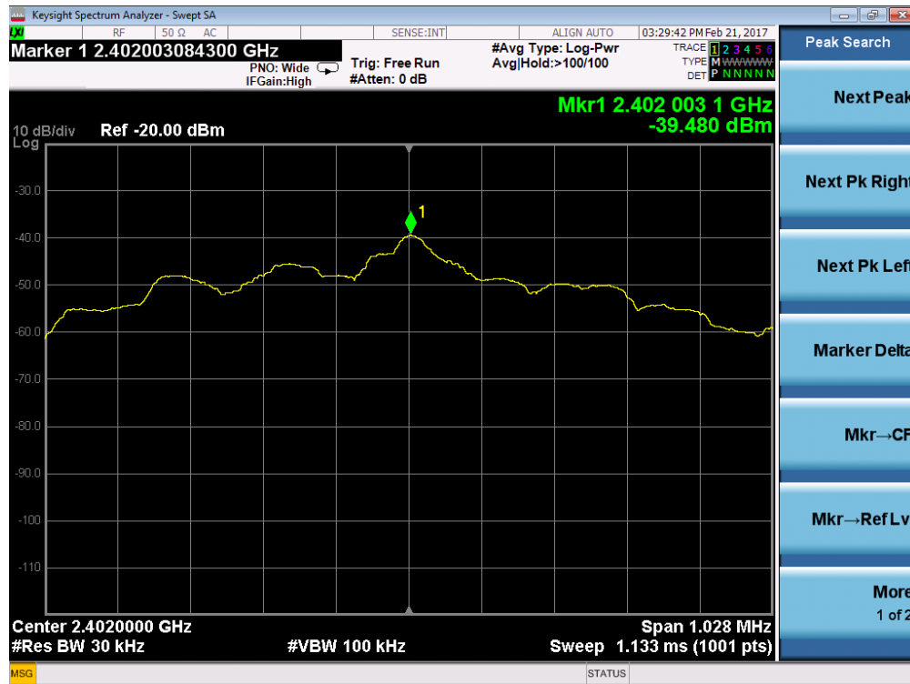
Low Channel Power Spectral Density
