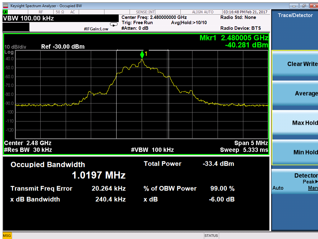
Occupied Bandwidth High Channel
