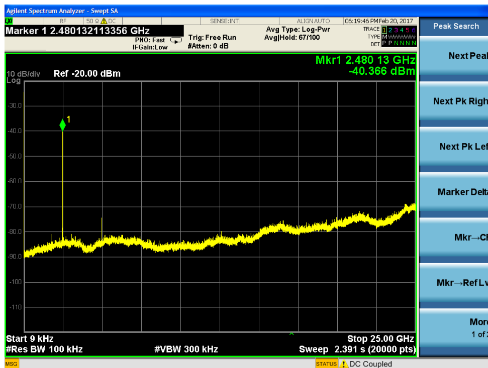
High Channel 9 KHz -25GHz Conducted Spurious
