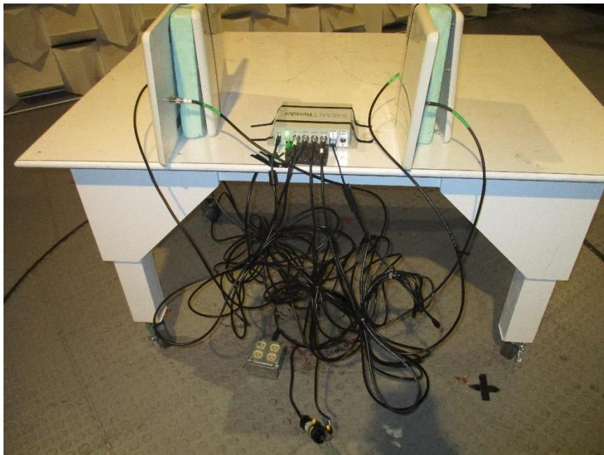
**Radiated Emissions****Test Setup****Wiring Layout**
