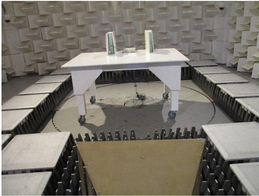
**Radiated Emissions****Test Setup****1GHz to 6GHz**
