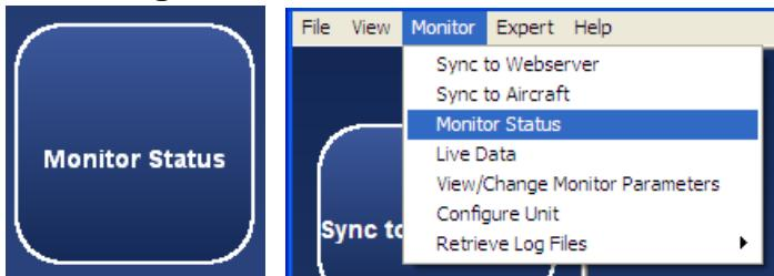
This function provides an overview of the status of the monitor and the status is updated continuously as long as the function is selected.
