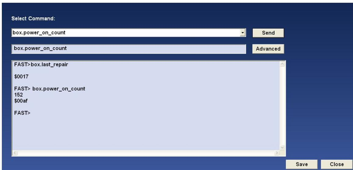
Selecting the Advanced button requires entering a password for advanced troubleshooting and permits typing any command. To obtain the password, contact P&WC Customer First center.
