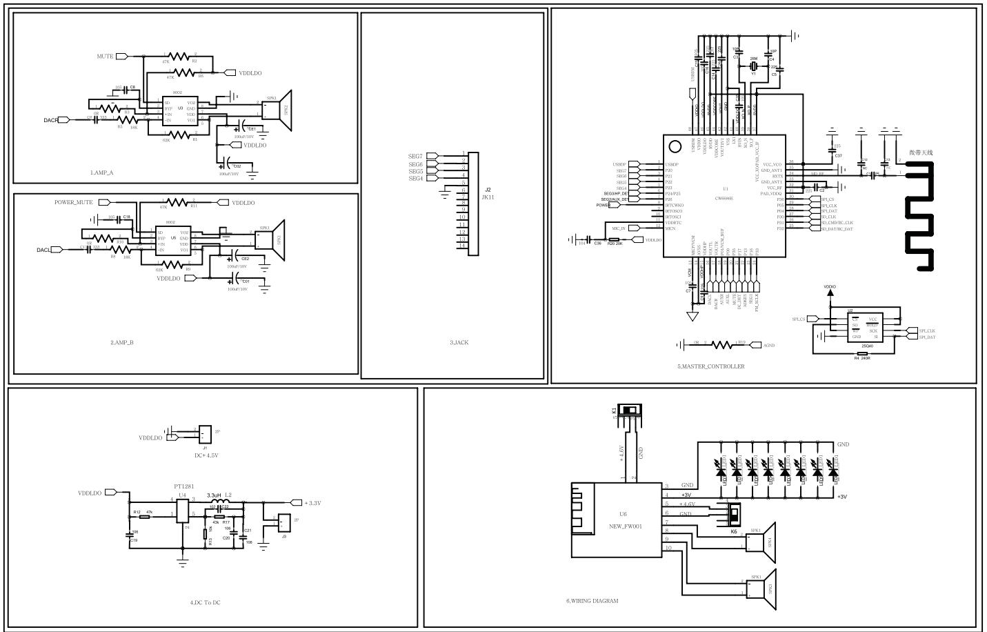
1, AMP\_A and 2, AMP\_B is power amplifier circuit
