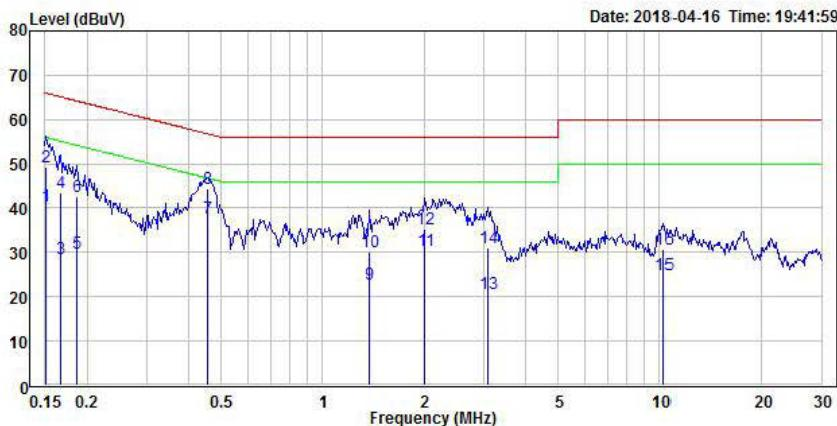
Condition: limit\FCC\FCC Conduction Clsaa-B QP.csv Neutral
