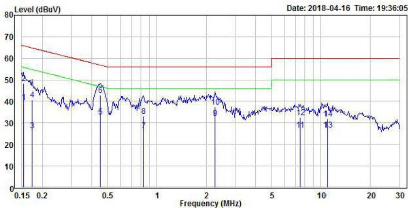
Condition: limit\FCC\FCC Conduction Clsaa-B QP.csv Line
