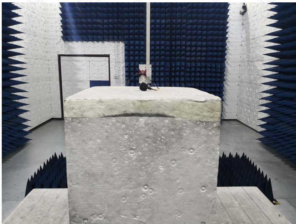
RADIATED EMISSION TEST SETUP ABOVE 1GHZ
