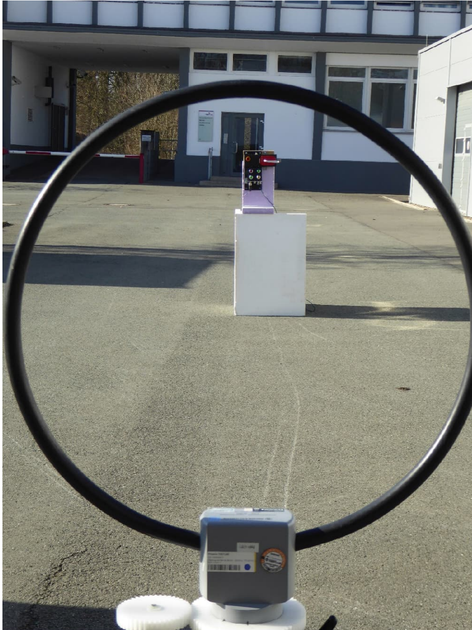
Test setup outdoor testsite (9 kHz to 30 MHz)
