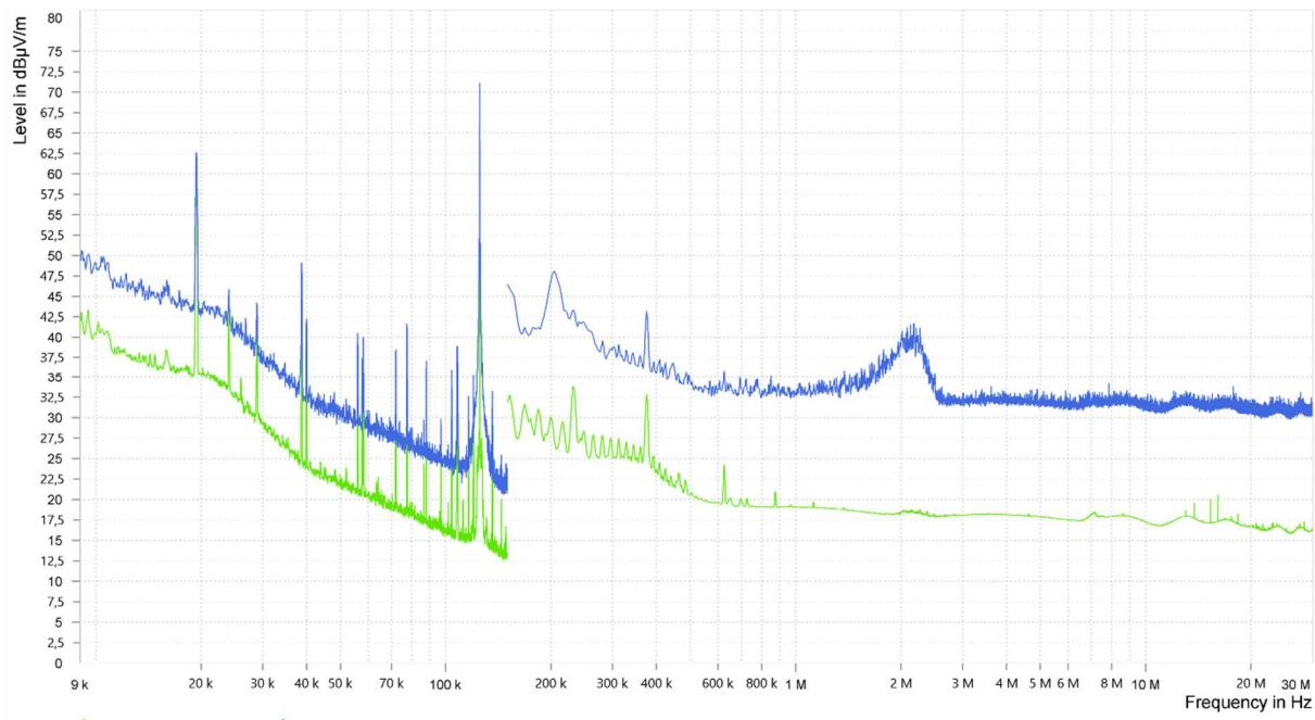
Only the fundamental of the transmitter (125 kHz) was found.
