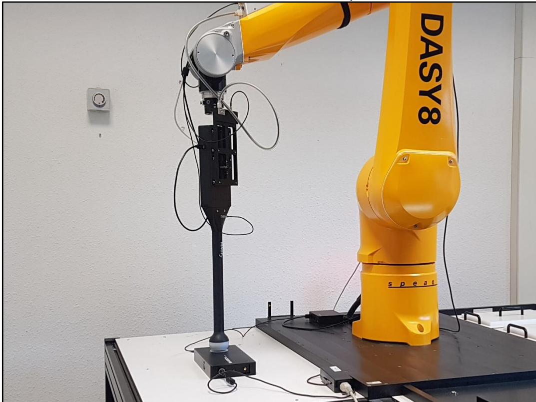
Photo 1: DASY 8 WPT set up
