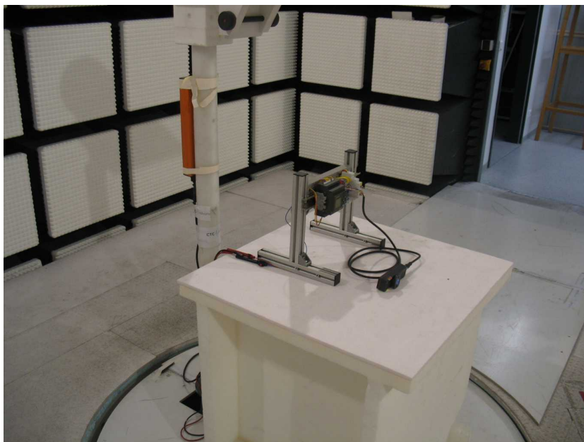
Photo 6: EUT at the anechoic chamber
