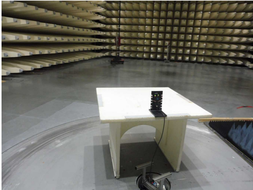
Photo 1: EUT at the semi-anechoic chamber
