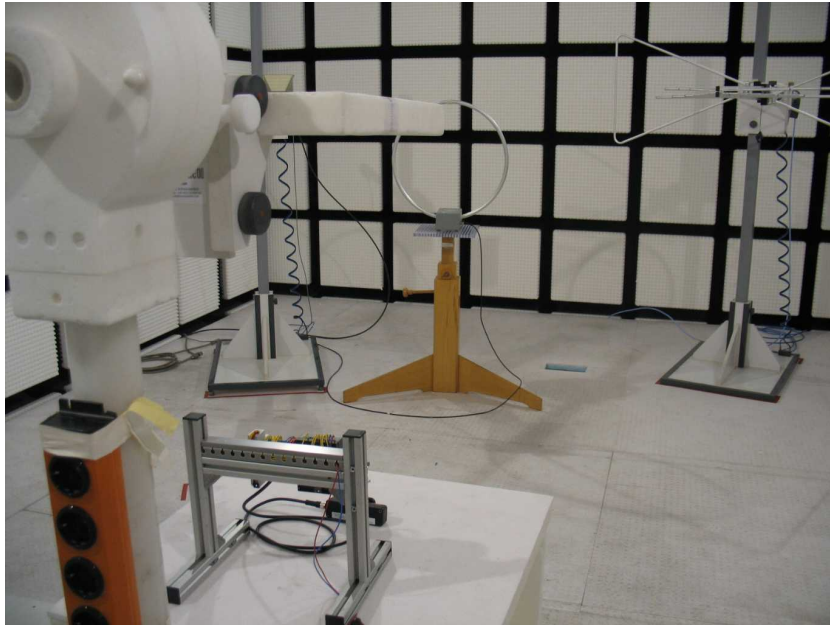
Photo 7: EUT at the anechoic chamber
