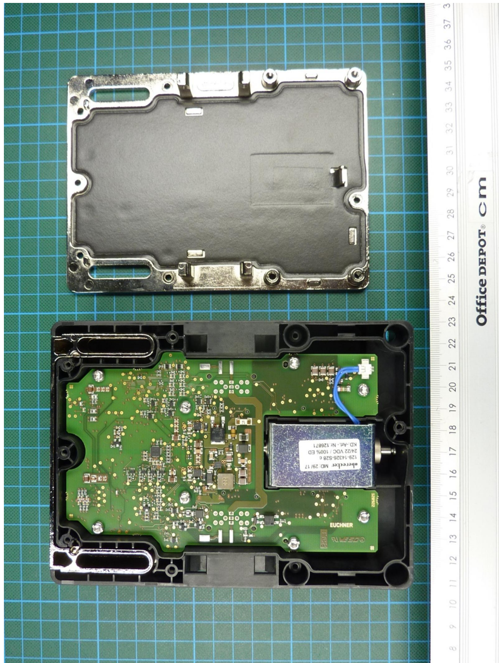
180889_19.jpg: MGB2-L1-MLI-U-Y0000-BJ-136776, internal view 2 (bottom cover removed)
