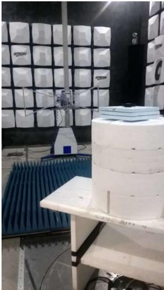
Radiated Spurious Emissions from 3 GHz to 18 GHz
