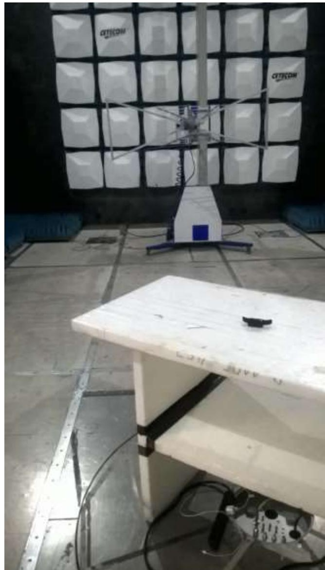
Radiated Spurious Emissions from 1 GHz to 3 GHz
