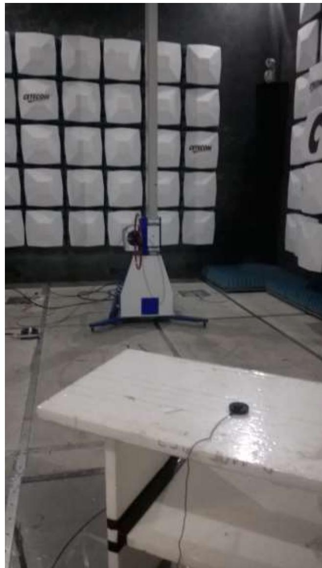
Radiated Spurious Emissions from 30 MHz to 1 GHz
