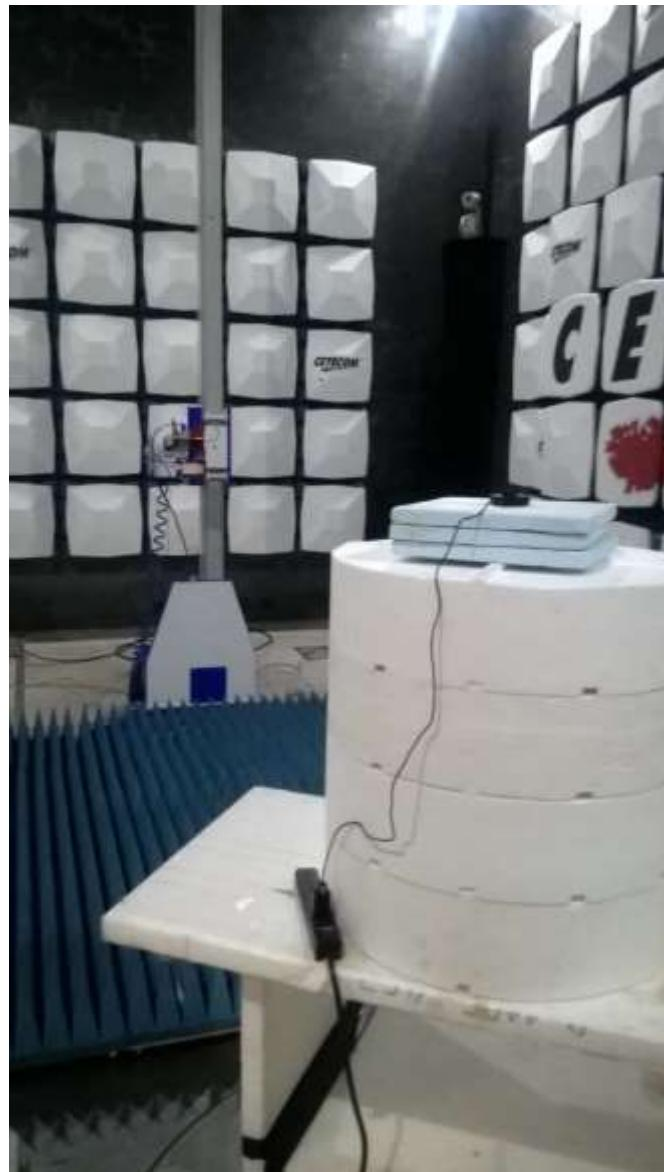
Radiated Spurious Emissions from 18 GHz to 26 GHz
