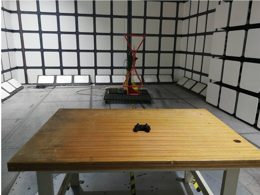
Radiated Emissions View (Below 1 GHz)
