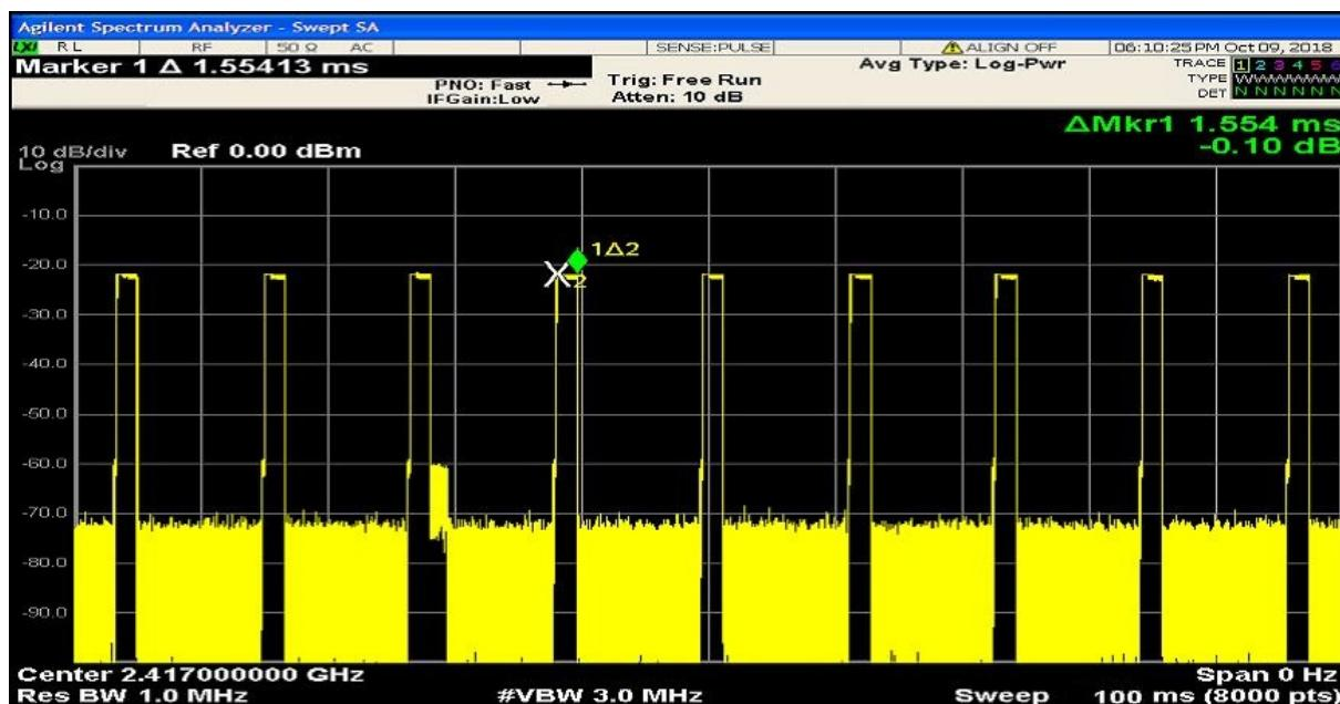
Mode:c; Polarization:Horizontal; Modulation:GFSK; ; Channel:Low
