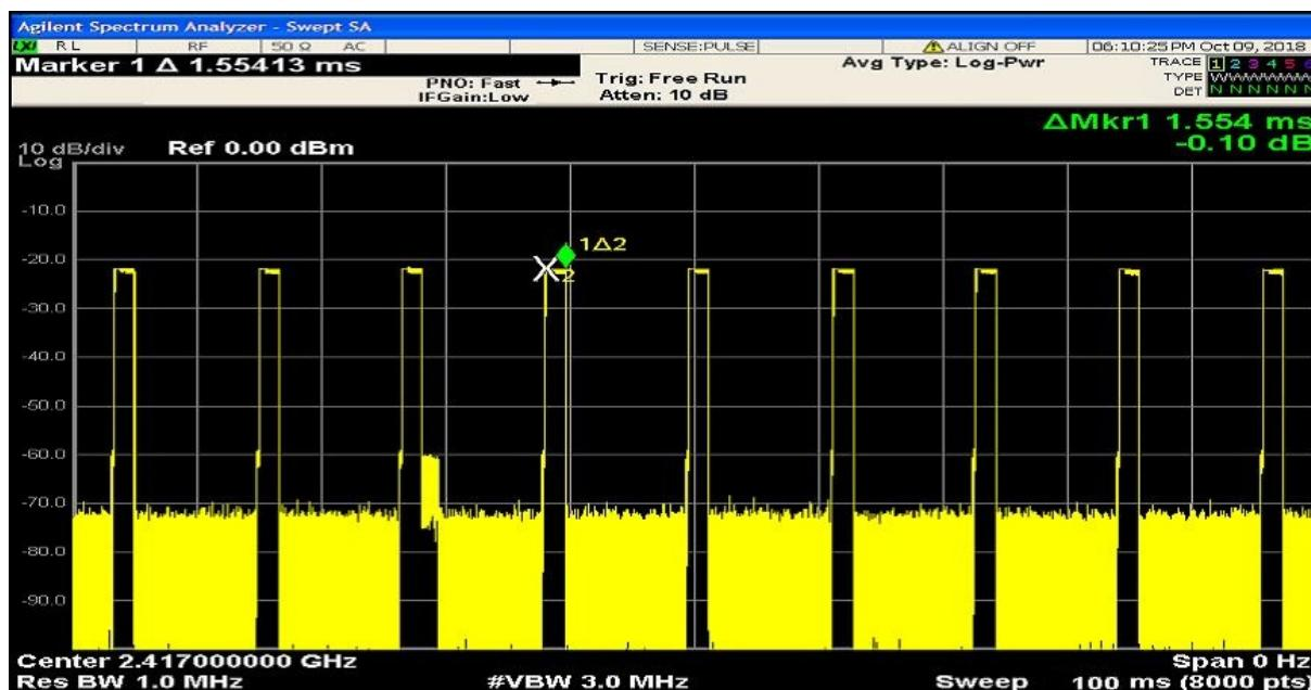
Mode:c; Polarization:Horizontal; Modulation:GFSK; ; Channel:Low
