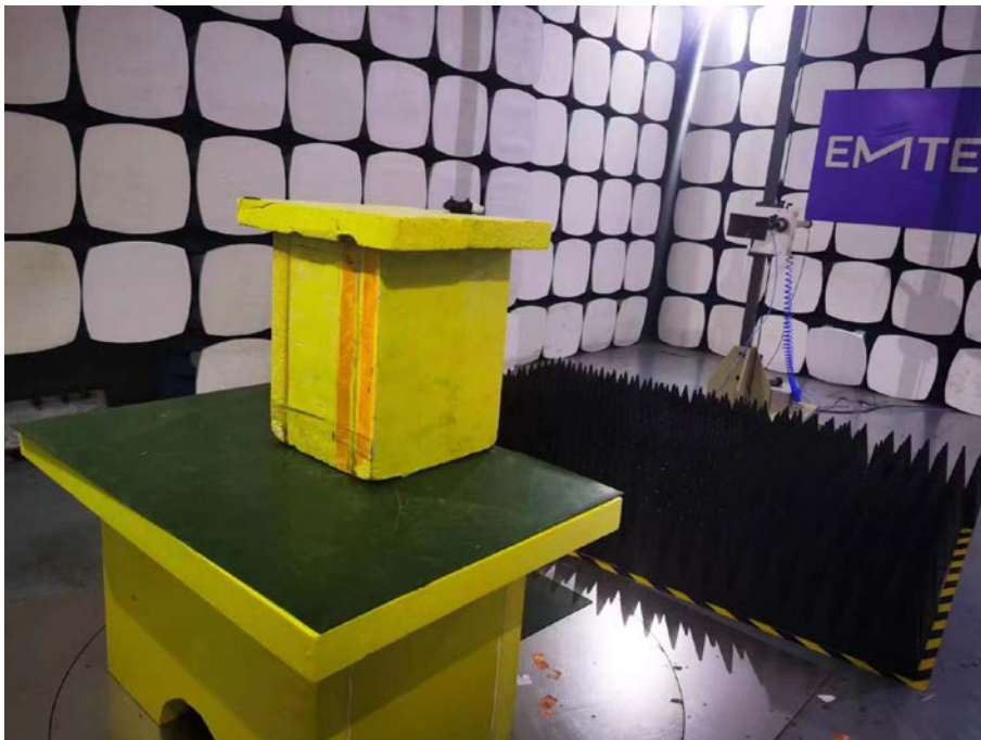
Spurious Emission Test Setup (Above 1GHz)
