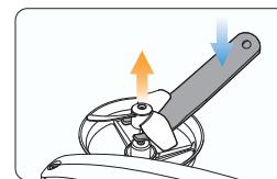
For propeller removal, Insert the propeller spanner between the propeller and the motor. Be sure to hold the motor while detaching the propeller.
