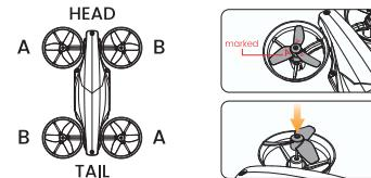
The drone will not fly unless the correct propeller is installed on the correct motor shaft. Each propeller is labeled with either an "A" or "B" on its. Install the propeller to the motor shaft and press into place.
