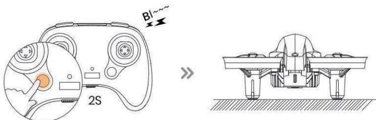
Make sure to place the drone on a level surface before calibrating the gyro. Long press the (
