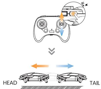
③ Wiggle Mode: The indicator lights on the drone will turn **solid purple**. The posture change is only visible **when the drone is flying forward or backward**.
