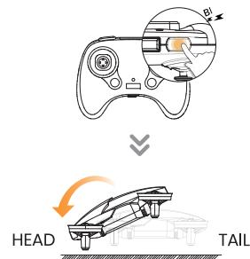
② Tilt Back Mode: The indicator lights on the drone will turn **solid blue**.
