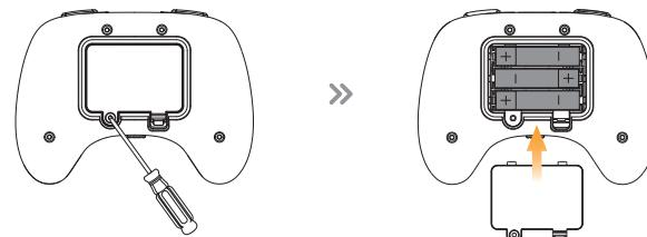
Open the battery cover on the back of the transmitter, insert the three AAA batteries (Not included) into the battery compartment. Then close the battery cover to complete the installation.
