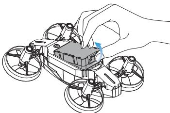
**⚠** The battery should be installed firmly. Otherwise, the flight safety of your drone may be affected. The drone may crash due to a power-cut during the flight.
