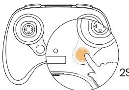
1 **Activating:** Long press the Headless Mode button ( ⌂ ). The transmitter will emit a continuous beep, indicating that the drone is in Headless Mode.
