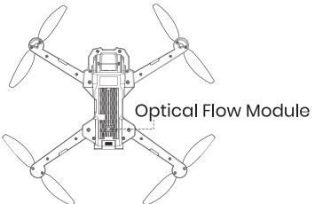
The Optical Flow Positioning System consists of a camera module, which acquires the position information of the drone through visual images to ensure precise positioning of the drone.
