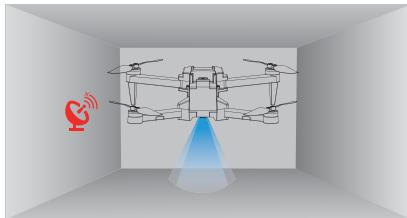
The Optical Flow Positioning System is typically used in an indoor environment when the GPS signal is weak or unavailable. The optimal usage height for Optical Flow Mode is **1.6-9.8 ft**.
