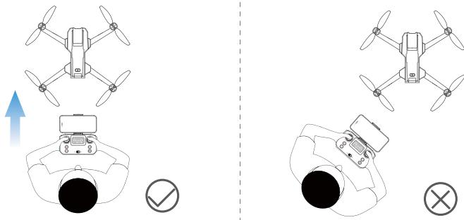
The pilot should stay facing the same direction that the drone's head points to when it takes off.
