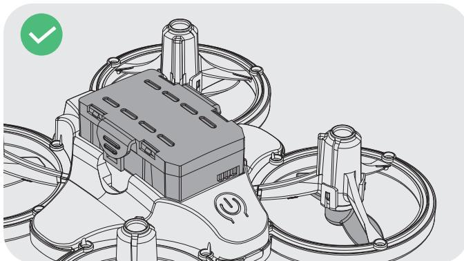
Make sure the drone battery and the propellers are mounted securely.
