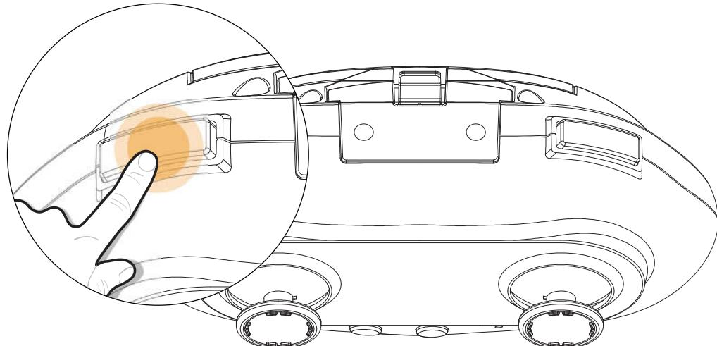
This drone comes with 2 speed modes (Low/High). Short press the
