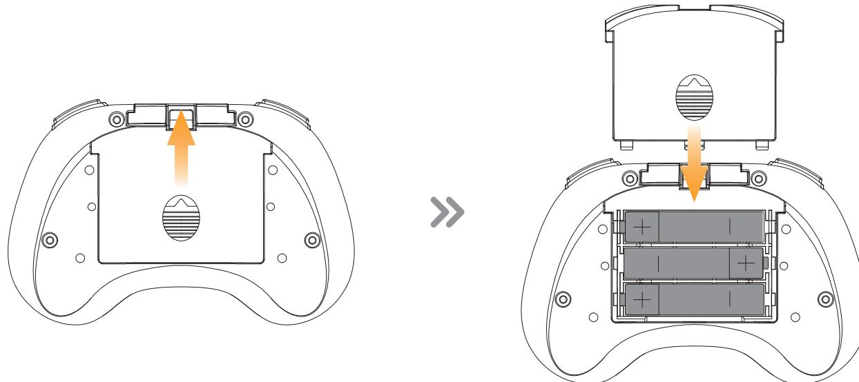
Open the battery cover on the back of the transmitter, insert the three AAA batteries (Not included) into the battery compartment. Then close the battery cover to complete the installation.
