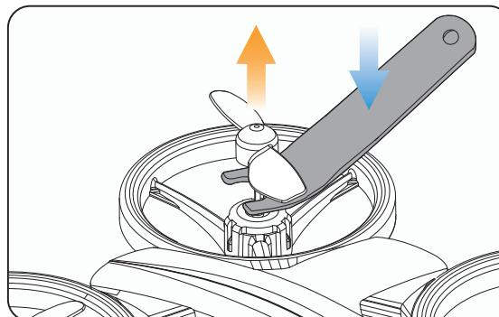
The drone will not fly unless the correct propeller is installed on the correct motor shaft. Each propeller is labeled with either an "A" or "B" on it. Install the propeller to the motor shaft and press into place.
